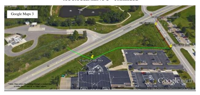
\*NOTE: Fiber enters the building through a conduit that is under the "i" and "b" in "Fiber" above.
